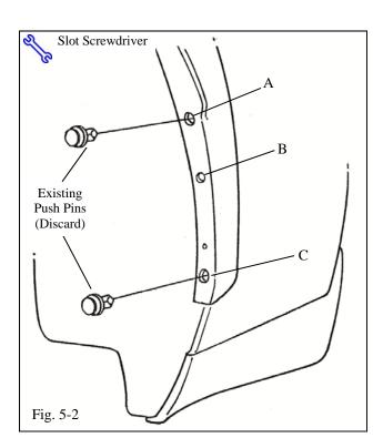
(c) Remove the existing push pins at locations A and C (Fig. 5-2). They will not be reused.
