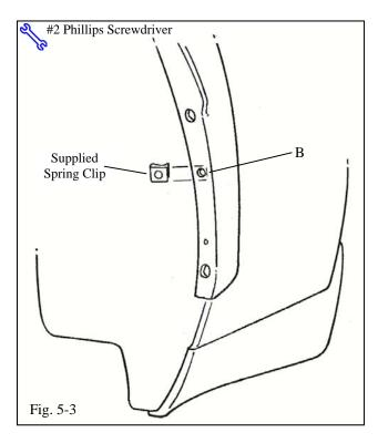
(d) Install a supplied spring clip over the panel edge at location B (drilled hole) (Fig. 5-3).
