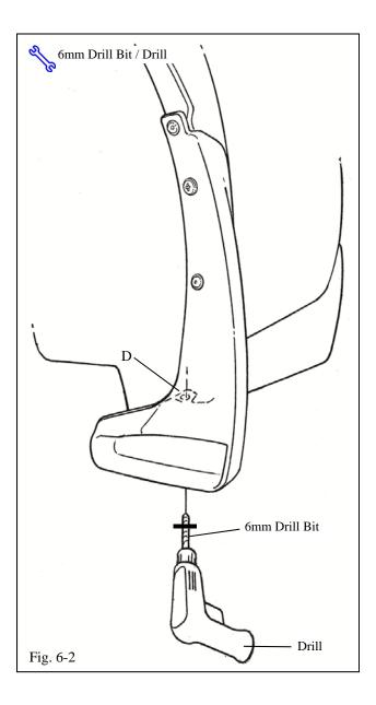
(c) With the drill stop still in place, hold the part up and into the bumper panel and use the part as a template to drill a 6mm (1/4") hole at location D (Fig. 6-2).
