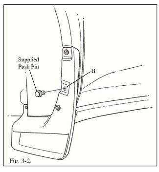
(c) Hold the part up and into the body panel and install a supplied push pin in location B (Fig. 3-2).
